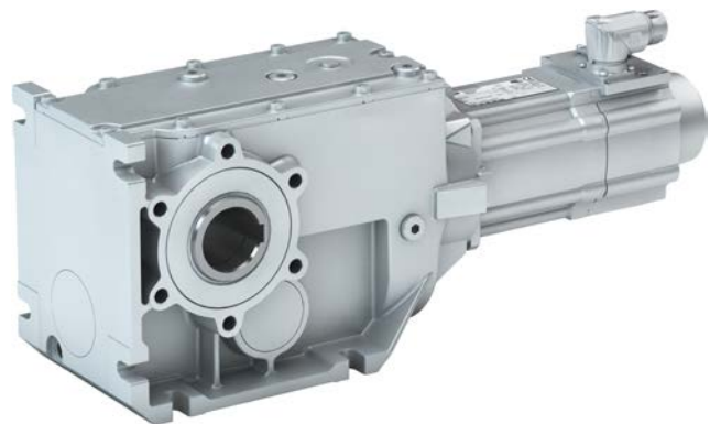
MCS09C synchronous servo motor - g500-B450 bevel gearbox with One Cable Technology (OCT) in connection with a digital absolute value encoder
