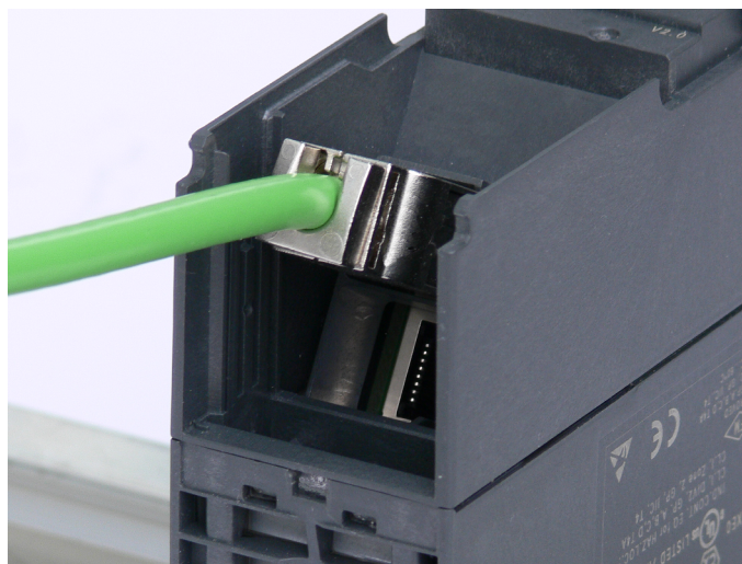
Figure 4-5 Inserting the IE FC RJ45 Plug 180
