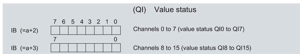
Figure 4-3 Address space for configuration as 16-channel DI 16x24VDC HS QI with value status
