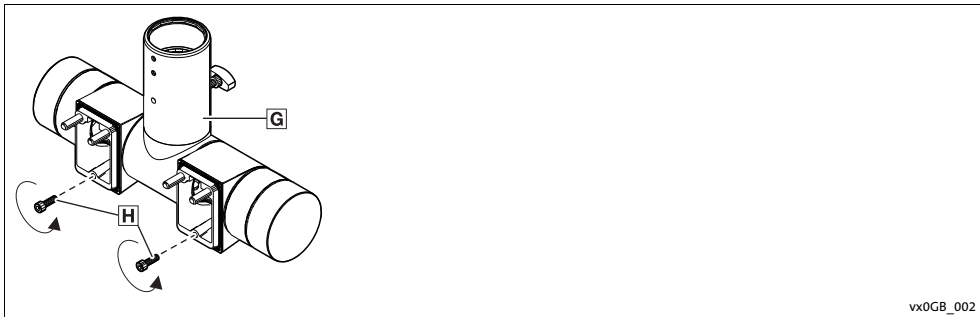
Fig. 2 Prepare the support arm adapter for mounting
