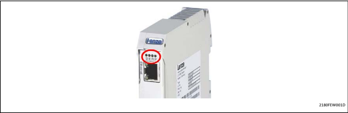
[8-1] LED status displays for the communication module and for CAN communication
