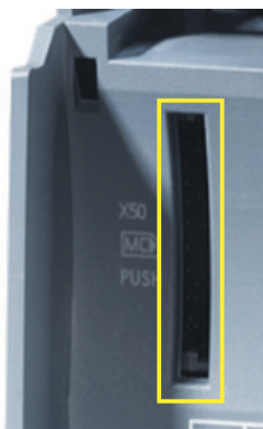
Figure 3-1 Slot for the SD card (yellow frame)
