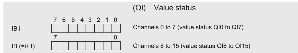
Figure 5-1 Address space for configuration as 16-channel DQ 16x24...48VUC/125VDC/0.5A ST with value status
