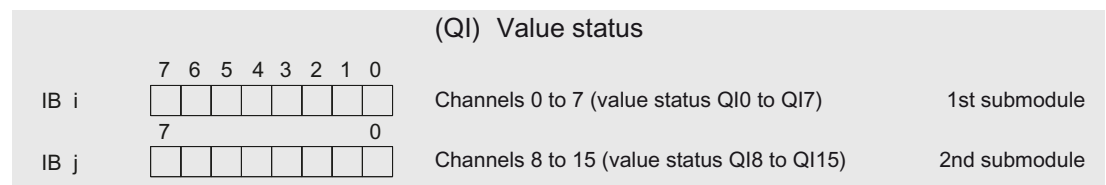
Figure 5-2 Address space for configuration as 2 x 8-channel DQ 16x24...48VUC/125VDC/0.5A ST S QI with value status
