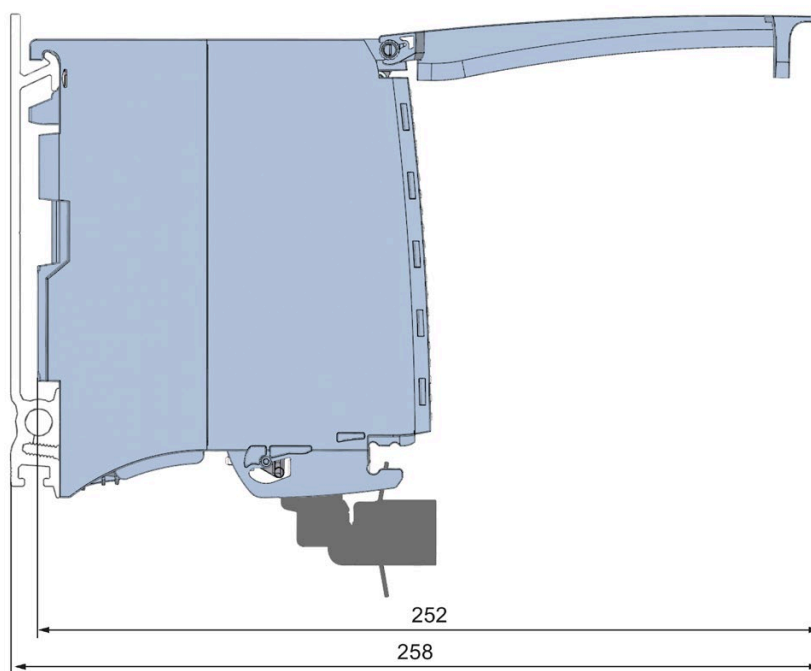
Figure A-2 Dimension drawing of the DI 16xNAMUR HF module in side view with open front cover
