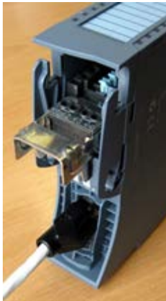
Figure 4-8 Ethernet cable connected to module
